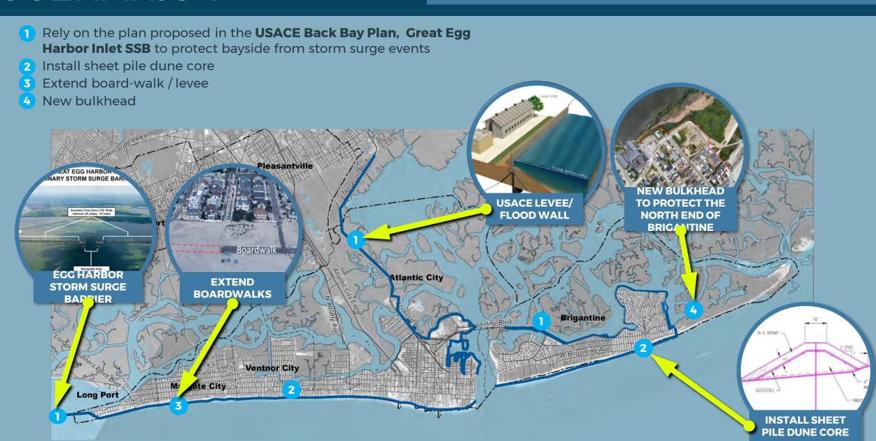
1 Rely on the plan proposed in the USACE Back Bay Plan, Great Egg **Harbor Inlet SSB** to protect bayside from storm surge events Install sheet pile dune core Extend board-walk / levee New bulkhead TO PROTECT THE **INSTALL SHEET NORTH END OF PILE DUNE CORE BRIGANTINE EXTEND BOARDWALKS AS EGG HARBOR** tic City **A CONTINUOUS** STORM SURGE BAPPIER Brigantine Brigantine Blvd **Ventnor City** gate City
