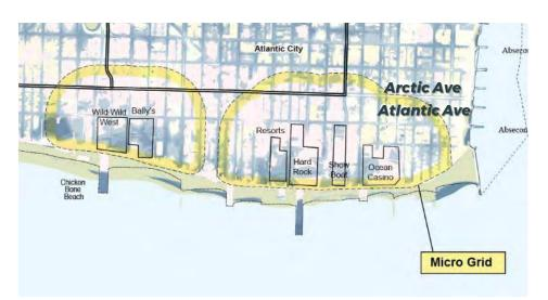
Coordinate with developer to expand microgrid to local merchants on **Atlantic Ave** that are critical after emergency events/outages.
